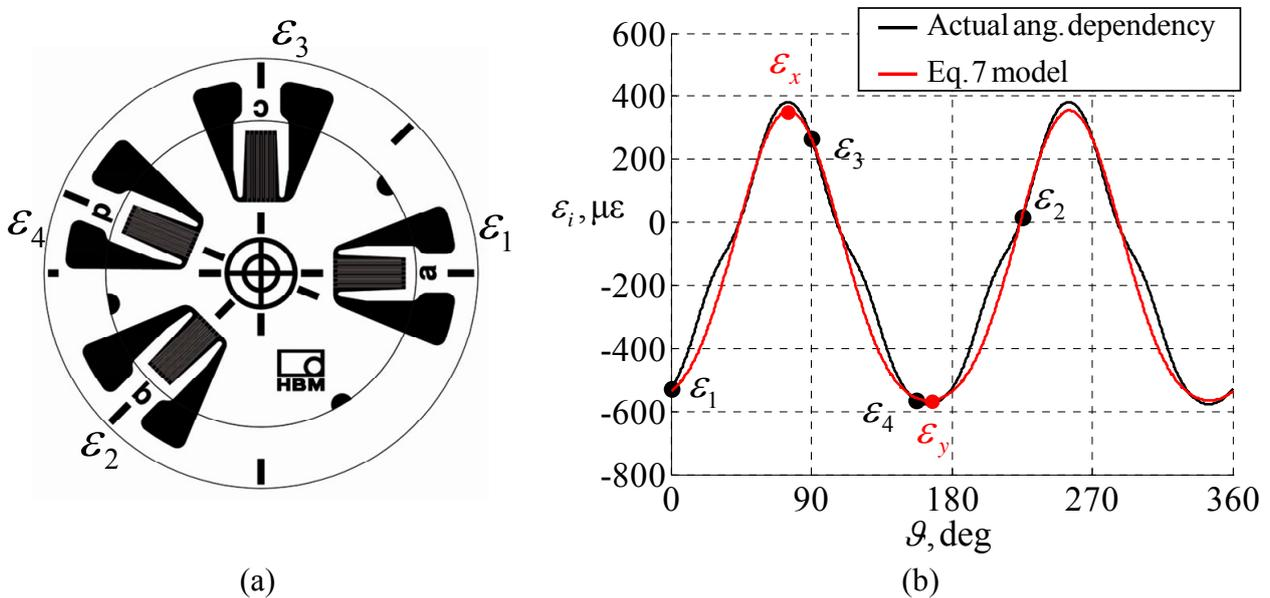
**Figure 4.** (a) Four grids rosette scheme. (b) Actual angular dependency and Eq. 7 model, determination of the residual stress principal directions relaxed strain components, from the model, after the four grids readings.
