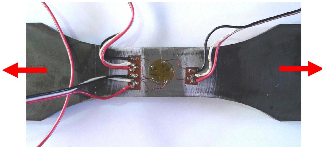
**Figure 5.** Experimental set up to simulate a residual stress by means of an external load.
