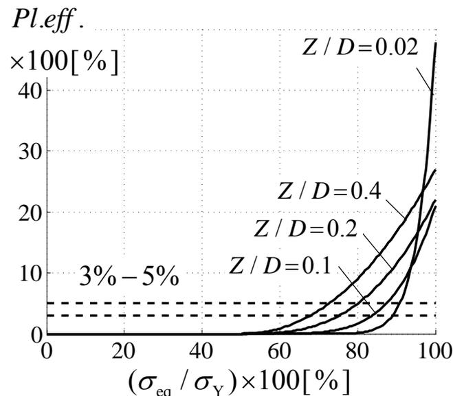
**Figure 2.** Plasticity effect intensity as function of the equivalent residual stress to material yield stress ratio.
