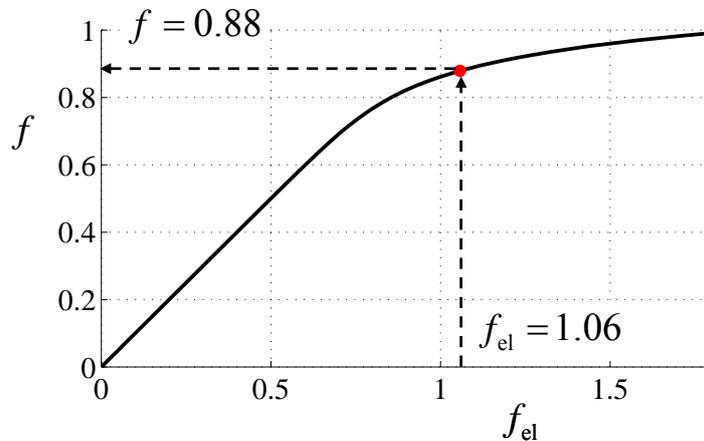
**Figure 3.** Relationship between the as elastic plasticity factor and the actual plasticity factor.
