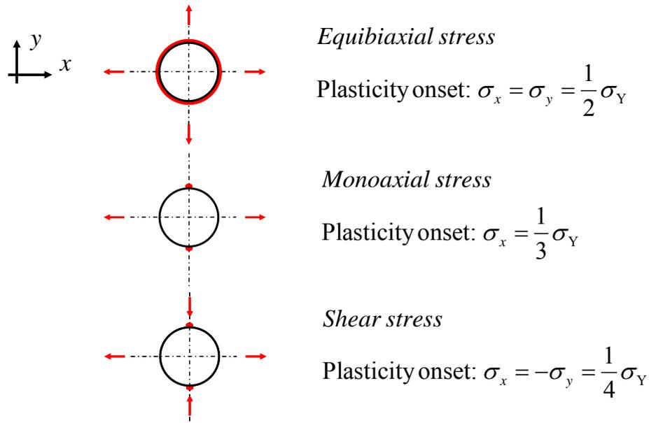
**Figure 1.** Plasticity onset limits, according to the plane stress Kirsch solution.
