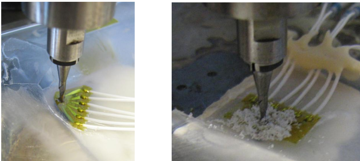
Figure 13. Drilling steps during the tests conducted with polycarbonate.
